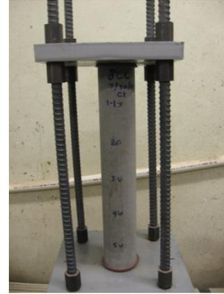
b.) Example Creep Cylinder Loaded in Creep Frame
