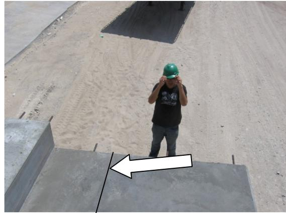
b.) Fishing Line with Tensile Strength of 0.22 kN (50 lbs) Tensioned at CGC on Left Side of HSC Beam
