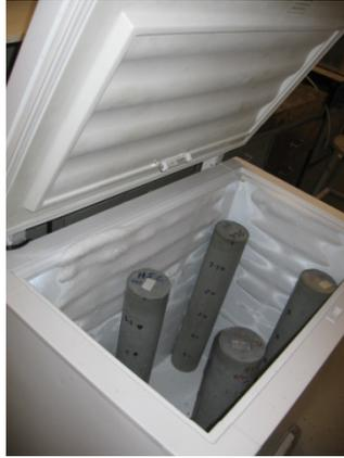
Figure 5.10. Coefficient of Thermal Expansion (CTE) Test at Missouri S&T.
