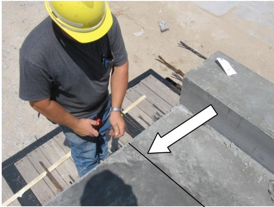
a.) Fishing Line with Tensile Strength of 0.22 kN (50 lbs) Tensioned at CGC on Right Side of HSC Beam
