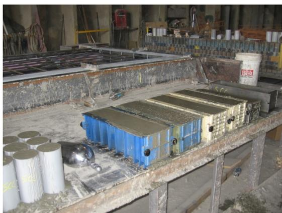
a.) Precast Spandrel Beam QC/QA Specimens
