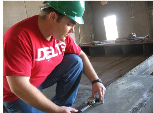
b.) DEMEC Reading with Gauge
