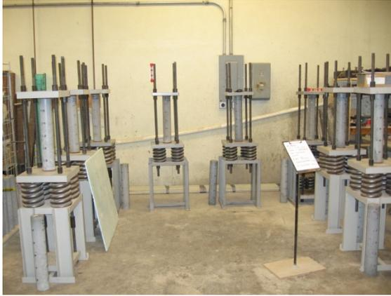
a.) Creep Frames at ERL Structural Engineering Laboratory
