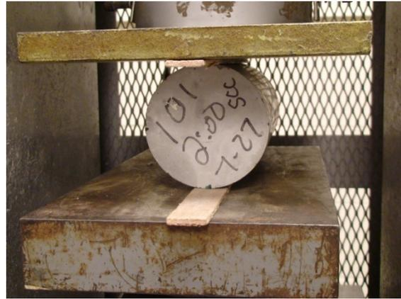
b.) Modified Split Tension Load Frame
