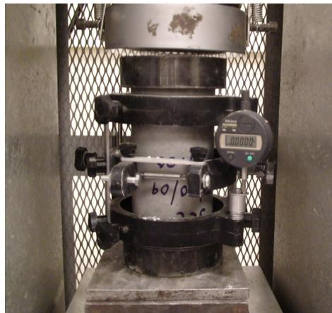
Figure 5.4. Modulus of Elasticity Test.
